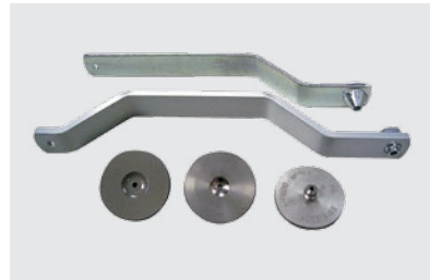
Top: Conical drilling jig, centre: drilling jig for hole = \varnothing 8.5 mm, bottom: rivet attachment jigs for rivet head dia. 11 and 14 mm mountable on riveting tool AccuBird (MBE)
