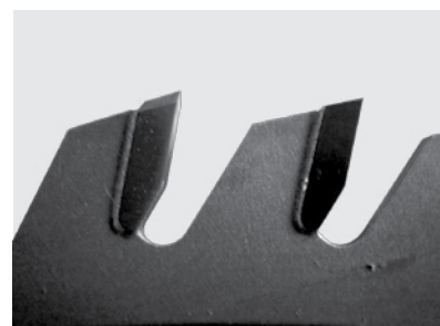
Tooth geometry trapezoid/flat tooth
